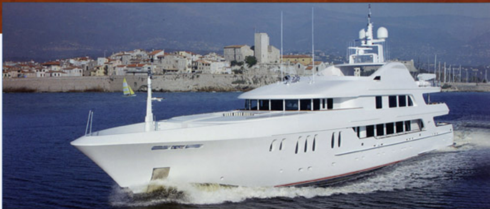
MUSTIQUE: Ex. Mia Elise 180' (54.8m) Tri-Deck Steel Hull/Aluminum Superstructure M/Y Naval Architect: Trinity Yachts, LLC Exterior Stylist: Trinity Yachts, LLC Interior Designer: Dee Robinson Interiors
